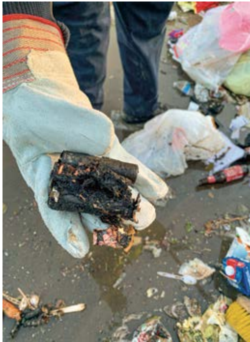
This lithium-ion battery pack was most likely to blame for a fire in a trash collection truck that required the load to be emptied onto a street so the fire could be put out.
